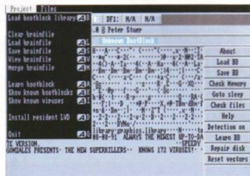
BootX is excellent for checking different boot blocks, and can also record the boot blocks from commercial game disks – a useful back-up if a nasty virus overwrites them.
